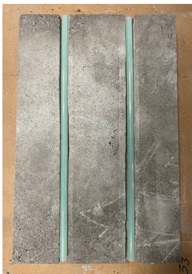
Milled sample with JK floorheating tube
