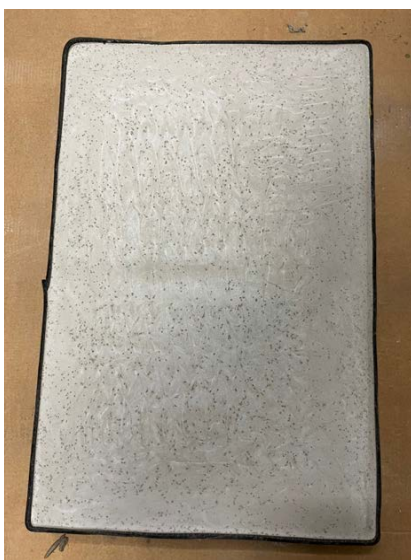
Leveling compound hardened
